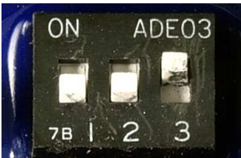
Map 2 : switch n. 3 (see photo). This is the map for the Polini engine Ø 44mm and Polini muffler.
