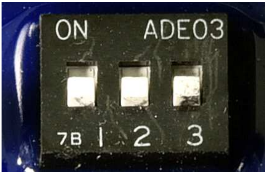
Map 2 : switch n. 3 (see photo). This is the map for the Polini engine Ø 44mm and Polini muffler.
