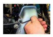
Refit the protection cover with the original screws.
